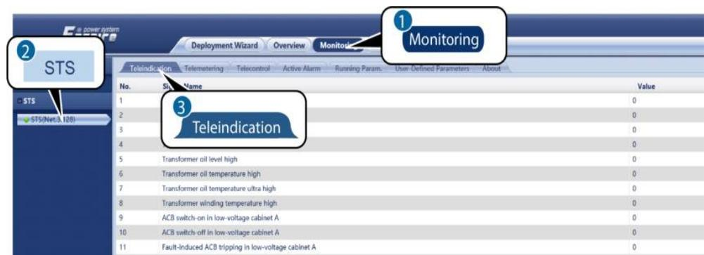
Figure 6-57 Viewing telemetry signal parameters
