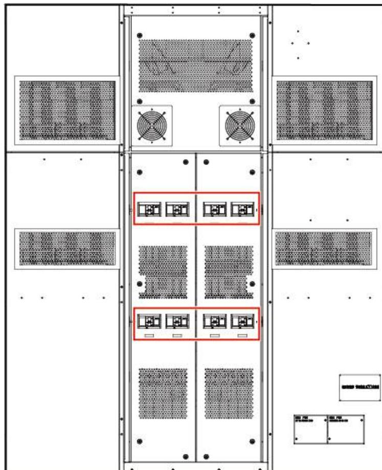
Figure 6-22 MCCB on the rear of the LV panel
