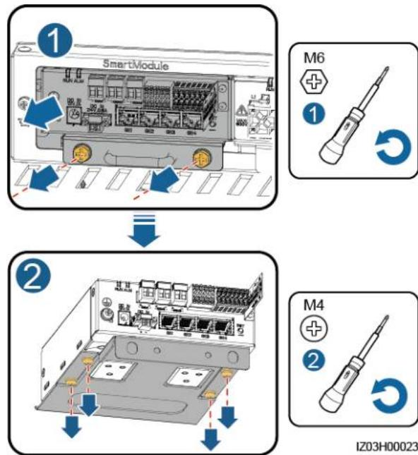
**Step 3** Remove the mounting ears and guide rail–mounting kit from a new SmartModule, and install the cabinet-mounting kit.
