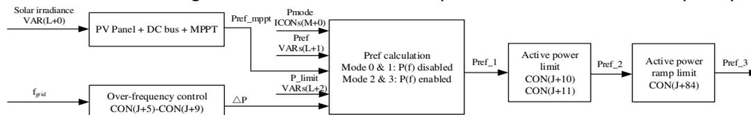
Figure 2: Active power management with over-frequency control
