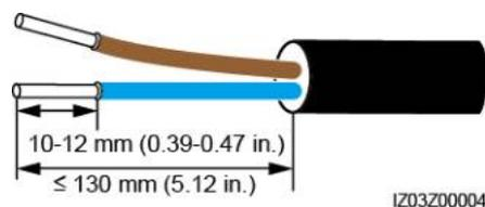
**Step 2** Connect the cable to the single-phase input switch.
