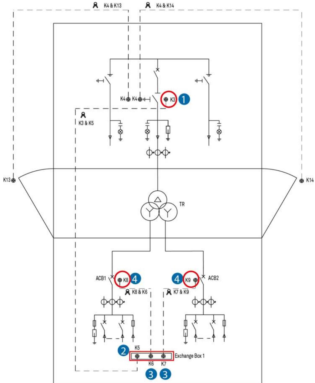
**Figure 4-13** Interlock inside the LV room (method 2)
