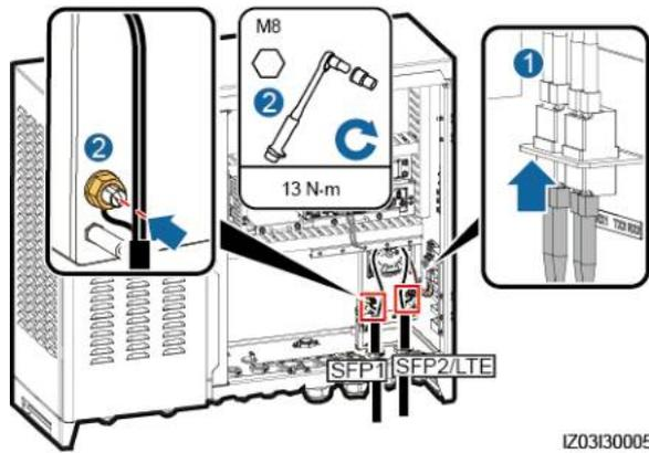
**Step 6** Check that the cables are connected correctly and securely. Then reinstall the optical cable fastener and external mechanical parts.
