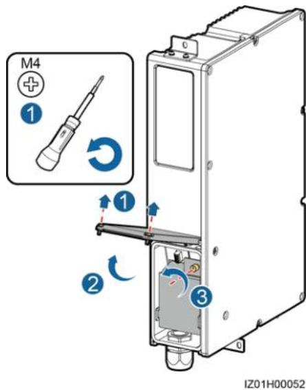
**Step 3** Disconnect cables from the faulty PID module, and label the cables.
