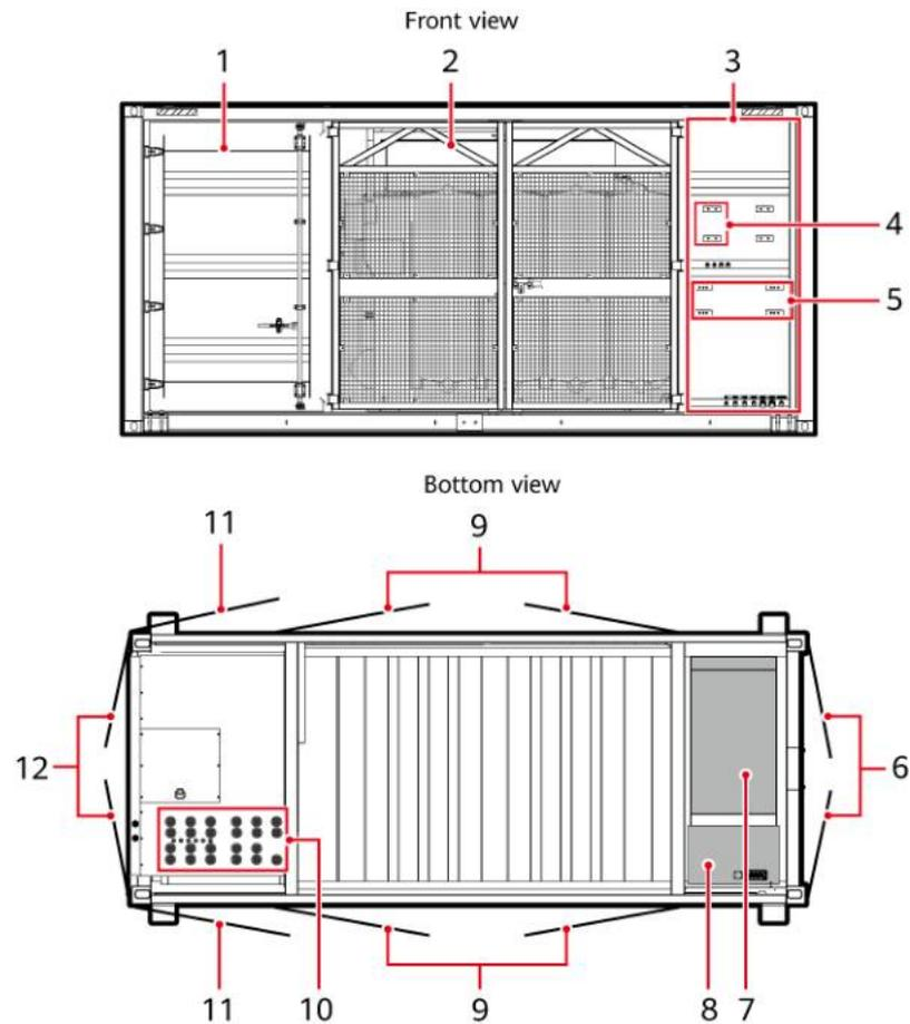
**Figure 2-7** JUPITER-6000K-H1 exterior (LV coupling scenario where the inverter and PCS are connected to the same MCCB)
