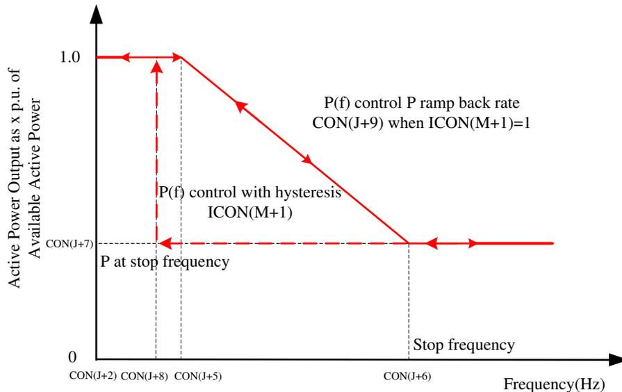
Figure 3: Over-frequency control
