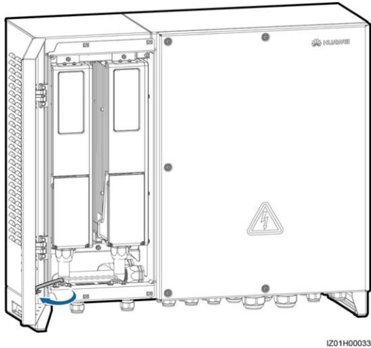
**Step 2** Open the maintenance compartment door of the PID module, and remove the cover from the connection box.
