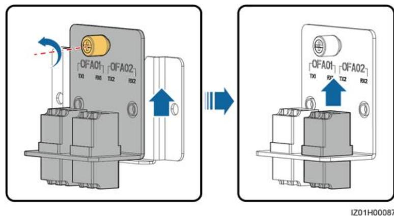
**Step 3** Install a new fiber adapter.
