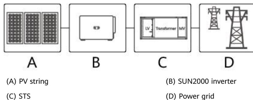
**Figure 2-2** LV coupling scenario where the inverter and PCS are connected to the same MCCB
