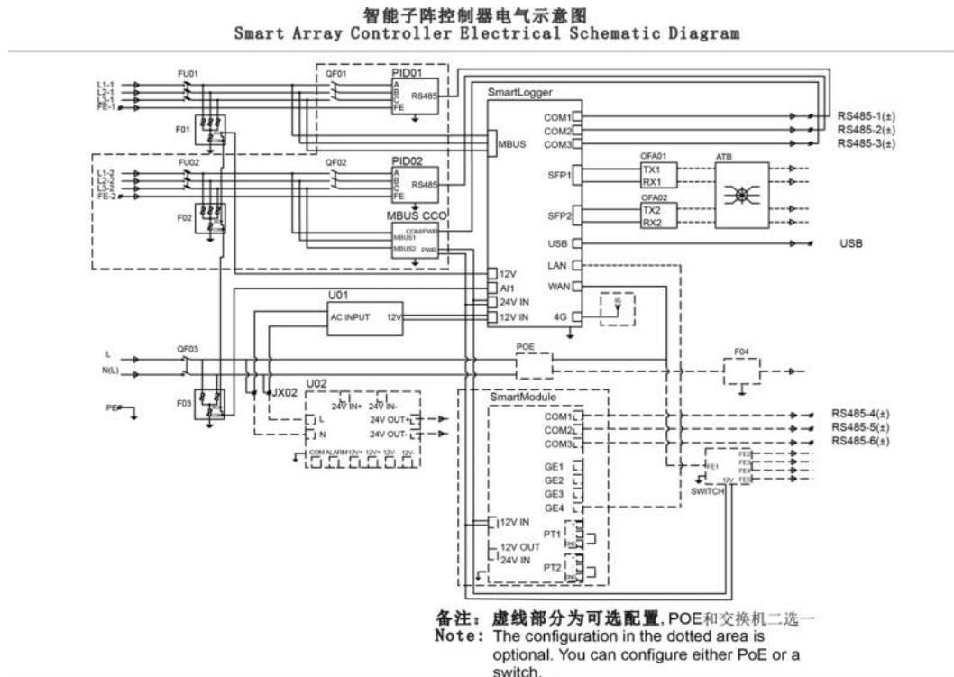
The SACU communicates with devices in a PV array over RS485, MBUS, or Ethernet.
