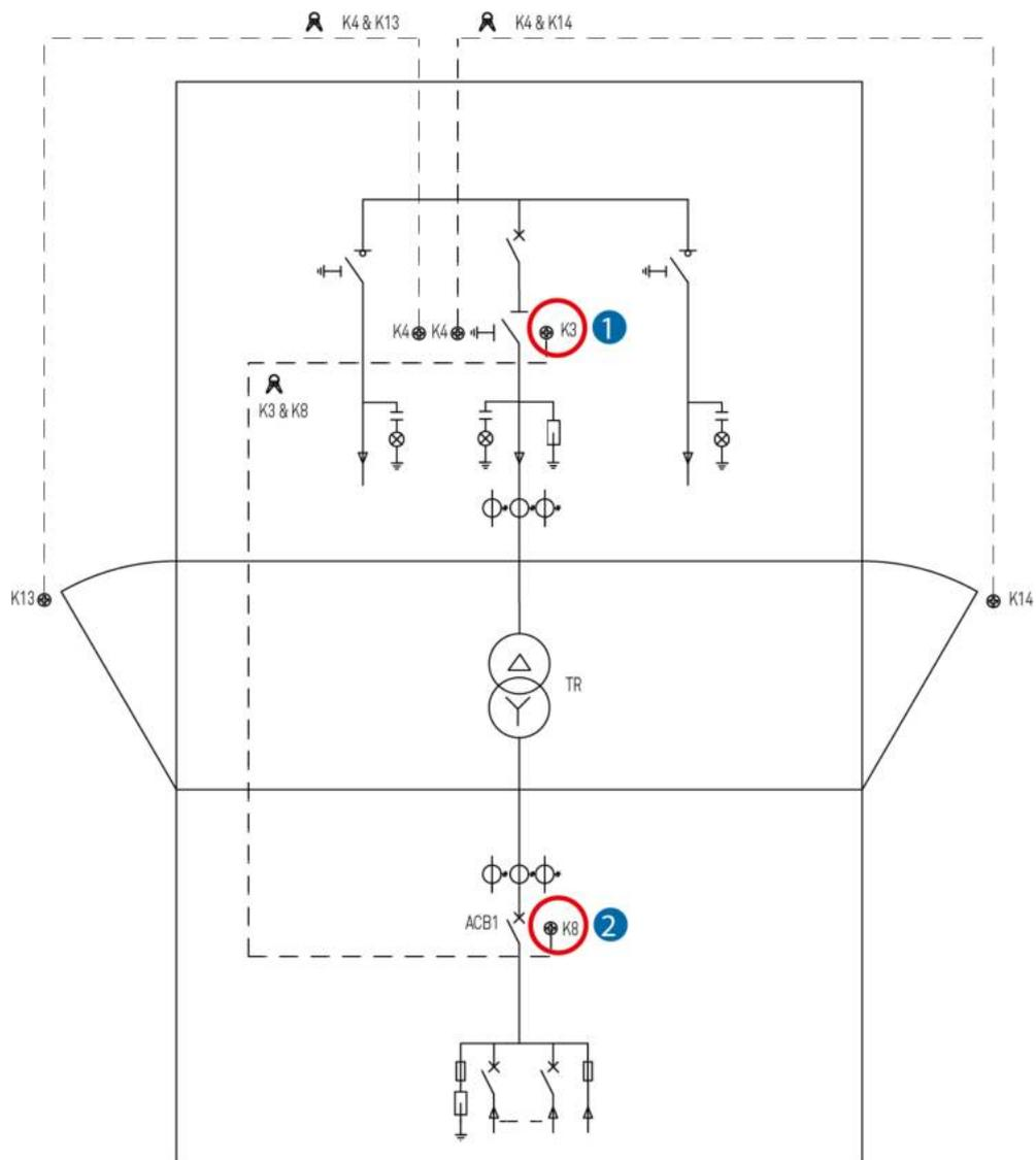
**Figure 4-15** Interlock inside the LV room (method 2)
