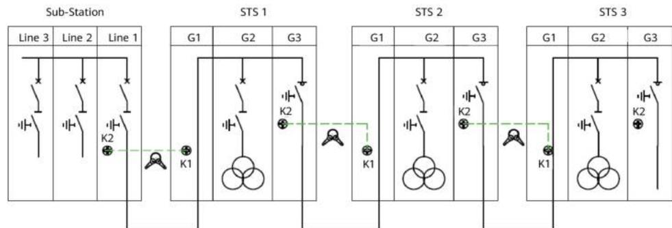
**Figure 4-10** Networking diagram of ring main units in DCV mode (8DJH series)
