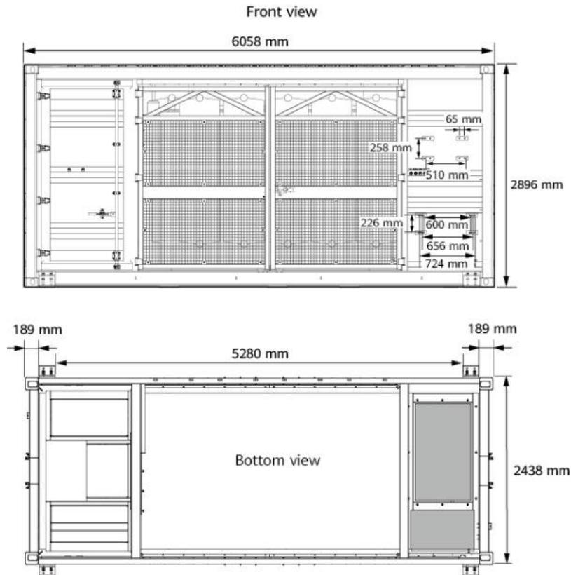
Figure 2-10 Dimensions of an anchor pad
