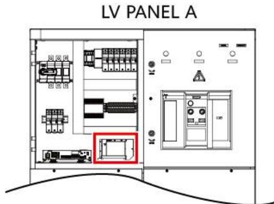
Figure 2-41 Appearance of the MBUS CCO
