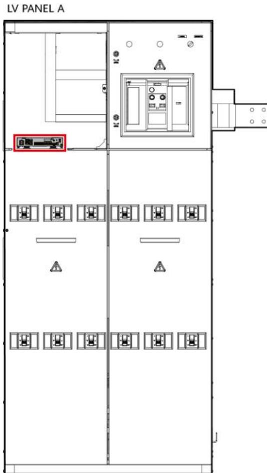
**Figure 2-34** Main control module (SmartMonitorA02)
