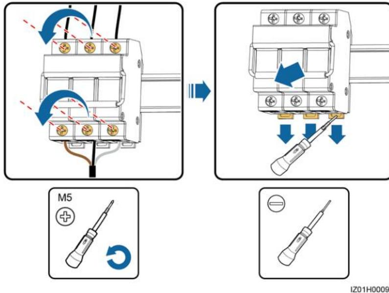
**Step 3** Install a new knife fuse switch.
