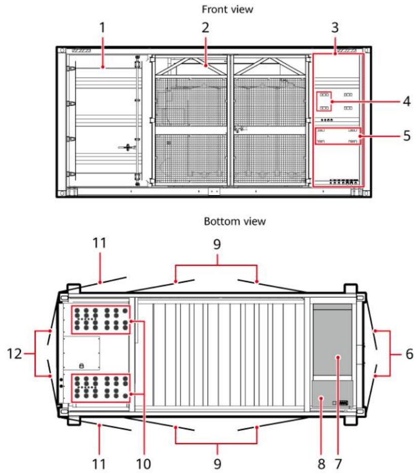
**Figure 2-8** JUPITER-9000K-H1 exterior (LV coupling scenario where the inverter and PCS are connected to the same MCCB)
