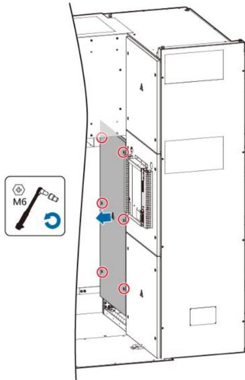
**Figure 6-44** Screws on the sealing plate of the JUPITER-9000K-H1 LV panel
