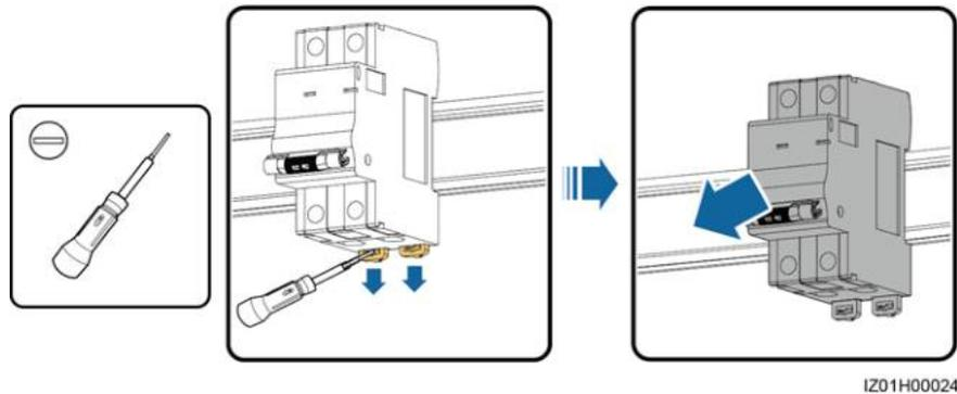
**Step 3** Install a new single-phase input switch.
