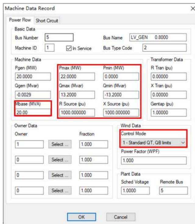
Figure 7: Machine setting
