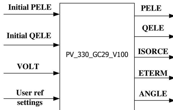
Figure 1 – Model input and output signals
