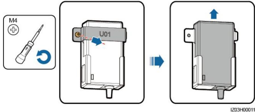
**Step 3** Install a new power adapter.
