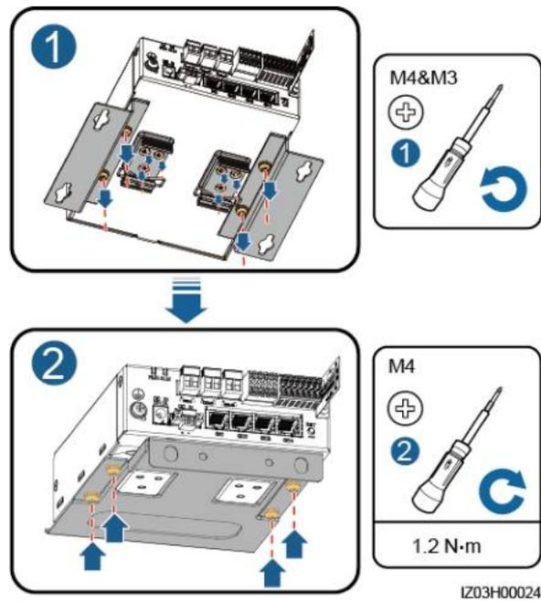
**Step 4** Install the new SmartModule in the cabinet.
