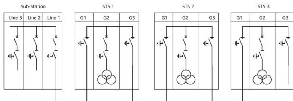
**Figure 4-7** Networking diagram of ring main units in CCV mode (8DJH series)
