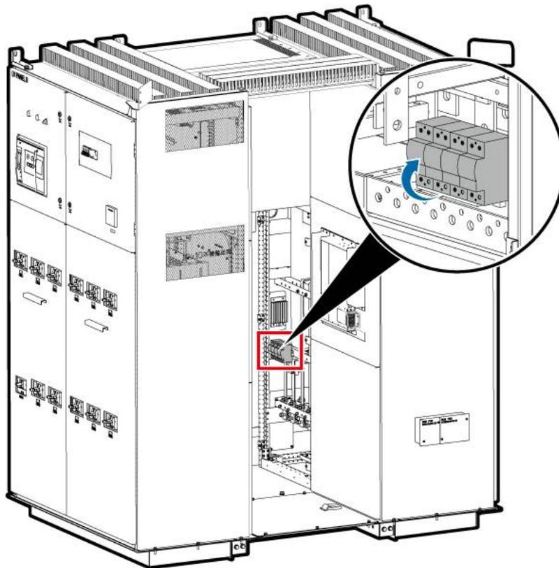
**Figure 6-26** Removing the SPD from the JUPITER-9000K-H1
