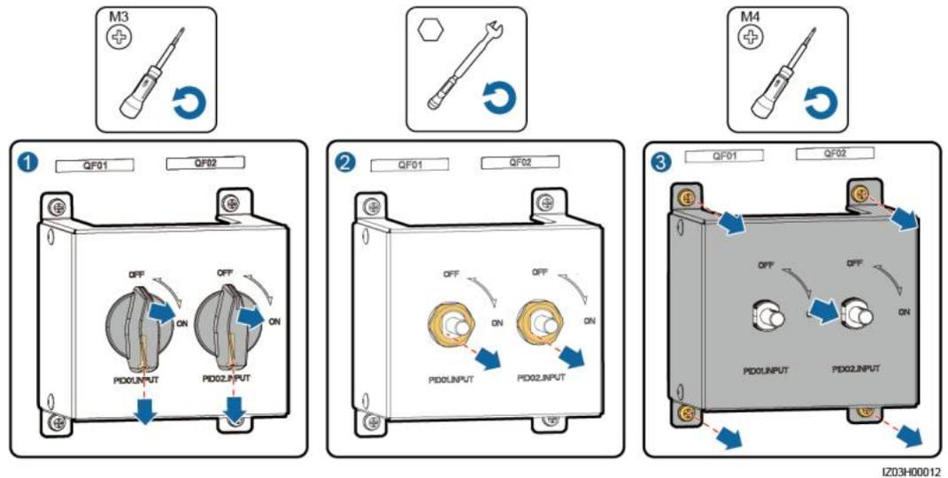
**Step 2** Disconnect cables from the switch of the faulty PID module, and label the cables.
